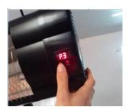
Step 6: After the function is on, 1-24 hours timing shutdown can be adjusted arbitrarily, the digital screen showing 0.1 indicates timing one hour, showing 0.2 indicates timing two hour.
